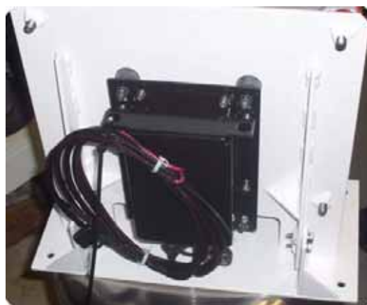
Figure 6. Haul truck mounting plate with BreadCrumb
